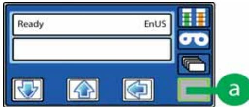
5. The USER button turns amber and **Menu available** displays on line 2. Press ENTER (b) to enter the menu system.
