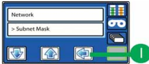
14. When you finish entering the subnet mask, **Network** displays on line 1 and **Gateway Address** displays on line 2. Press ENTER (m) and enter the gateway address, following the process in [step 12](#).
