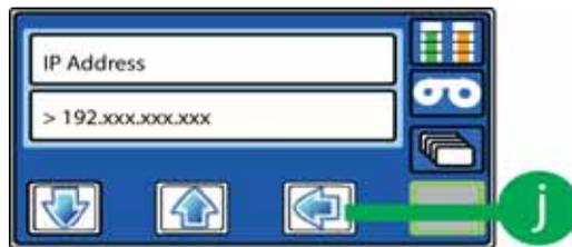
The address byte displays three digits when it can be changed.
