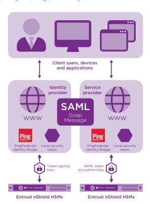
Entrust nShield Connect HSMs integrate with the PingFederate enterprise identity bridge to protect the SAML token signing and encryption keys within a high assurance environment, enabling keys to be exchanged between Web servers using Simple Object Access Protocol (SOAP).
