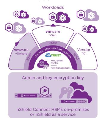
Entrust nShield hardware security modules (HSMs) secure the admin key and key encryption keys used to protect the HyTrust KeyControl key management server.
