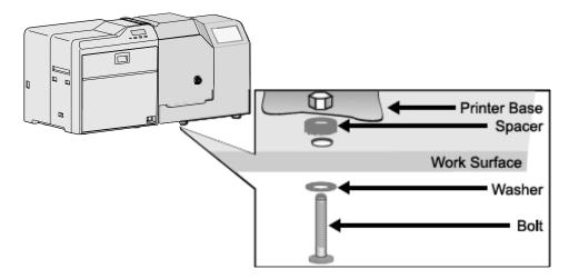
5. Turn the bolt into the rivet nut on the printer base, turning until the bolt is snug but does not cause distortion.
