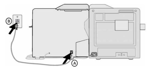
2. Connect the other end of the data cable to a network port (B).
