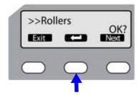
c. The **Film Checking** message displays, followed by **Cleaning Start OK?**. Press to start the cleaning process.
