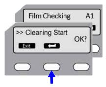
The print unit pulls the cleaning card into the print unit. **Cleaning** displays, and cleaning begins.
