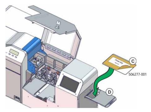
8. Insert the cleaning card into the exception card slide with the sticky side facing up. Push the card in until the end of the card rests in the slot (D).
